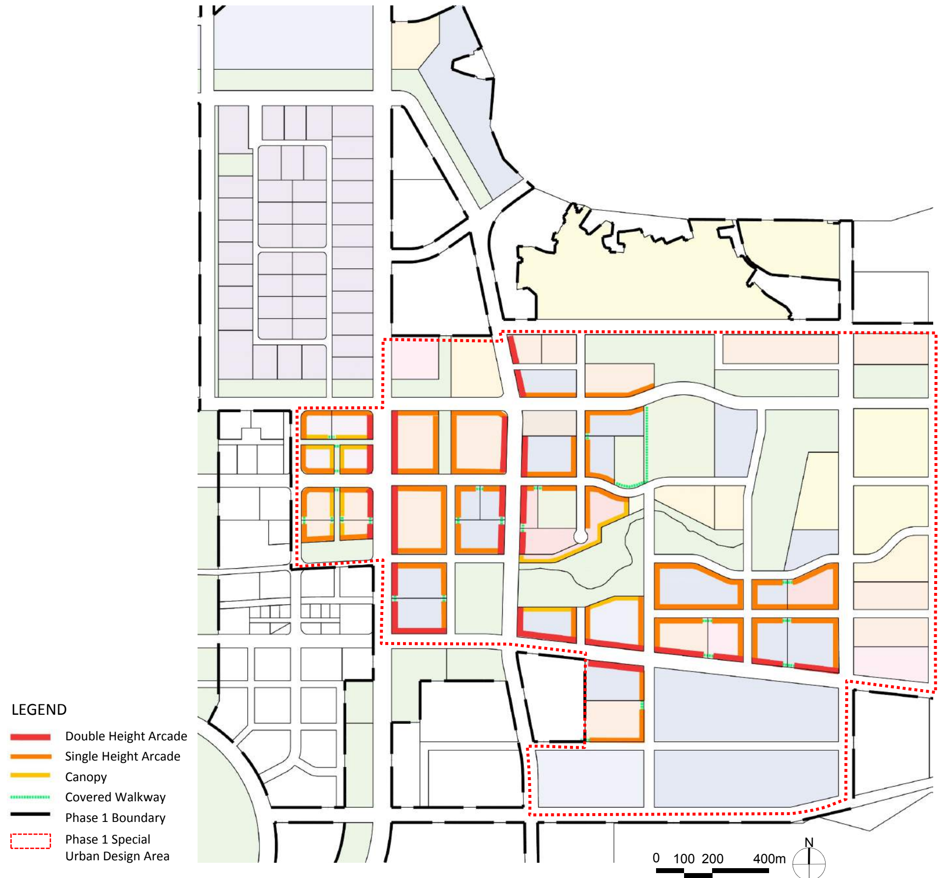
Fig. 5.8 Arcade, Canopy and Covered Walkway Plan
